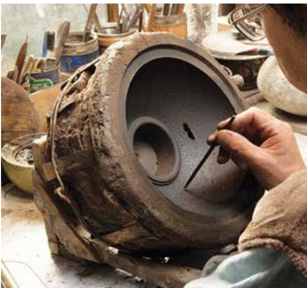
Fig 2. 'Grain pattern' using a spatula by hand
