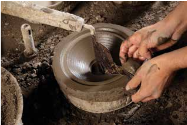
Fig 1. Rotate the template and make a mould with clay moulding sand
