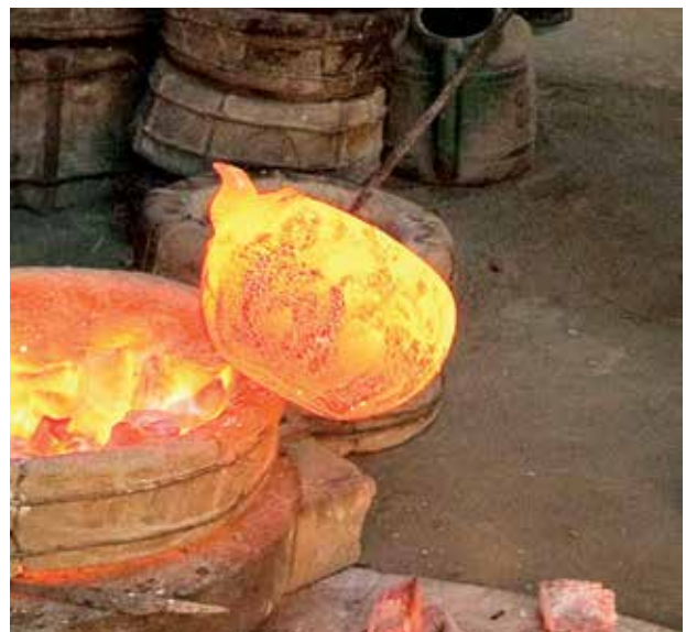
Fig 3. Heat treatment (distortion removal)
